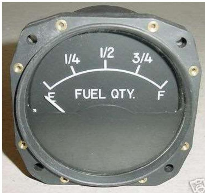
*flight. An indicator calibrated in appropriate units and clearly marked to indicate those units must be used. In addition: [ ] Each fuel quantity indicator must be calibrated to read "zero" during level flight when the quantity of fuel remaining in the tank is equal to the unusable fuel supply. . .*
