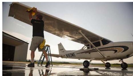
And remember not to use Simple Green All-Purpose Cleaner on aircraft, since it can promote corrosion if left on aircraft surfaces too long. Extreme Simple Green has been specifically formulated for use on aircraft.
