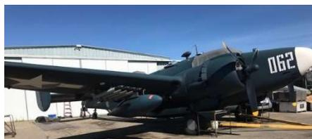
Sitting on the ramp outside Vintage Aircraft is a flyable PV-2D Harpoon. Used for maritime patrol, the aircraft had forward-firing machine guns, ball turrets and underwing rockets.
